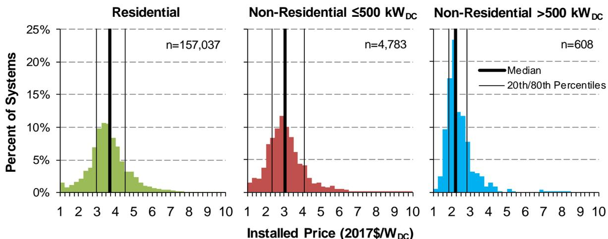
Figure 18. Installed Price Distributions for Systems Installed in 2017
